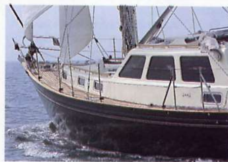
Above and left, high guardwires, plenty of handholds, bulwarks and sensibly proportioned side decks make her a secure boat to move about on
