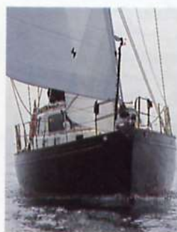
Above and left, high guardwires, plenty of handholds, bulwarks and sensibly proportioned side decks make her a secure boat to move about on
